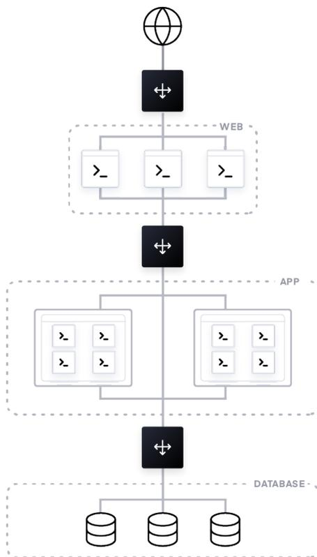
**Figure 2:** A static network topology with load balancers fronting the database, monolithic applications, and the web front-end.
