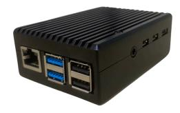
Plug the device into one of the access switches using an Ethernet cable and power up using a 5V power adapter.
