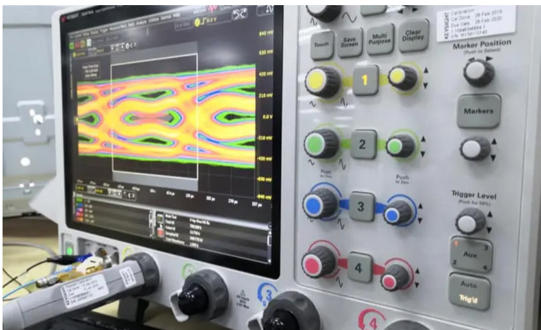
Figure 1: Oscilloscope eye diagram plot shows extreme jitter that includes ISI.
