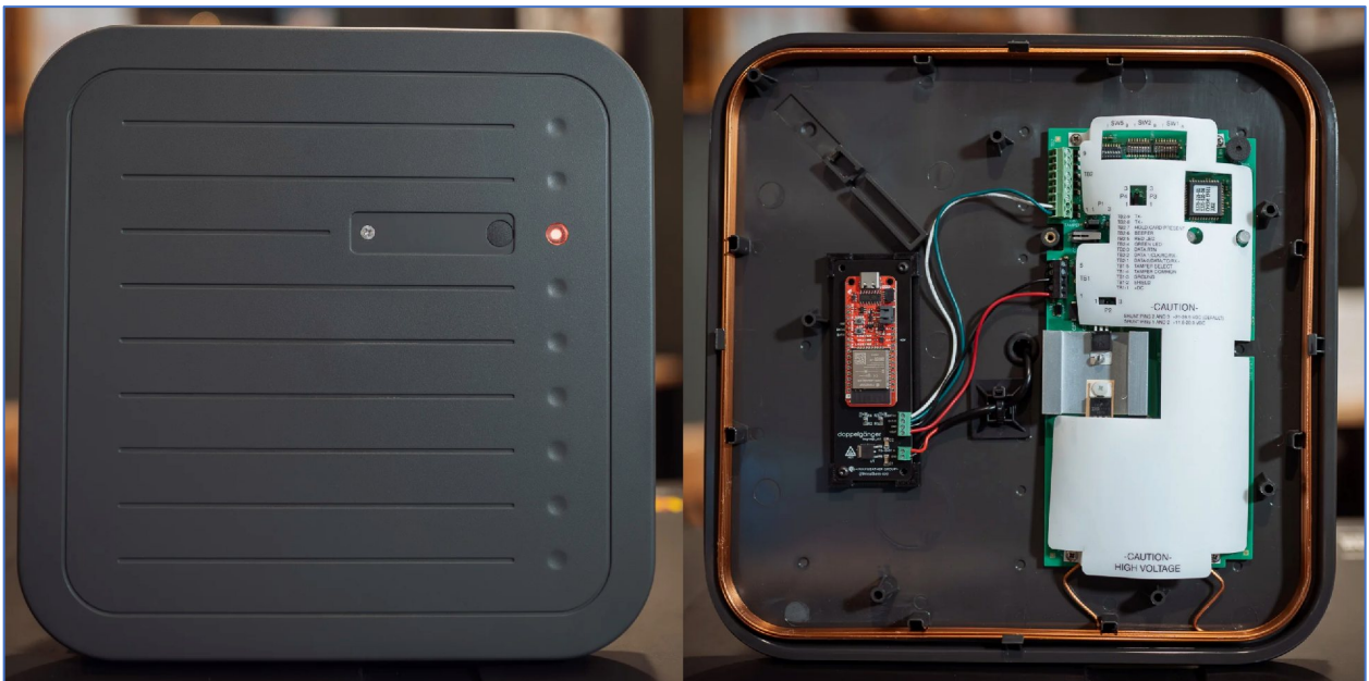
Figure 16: Doppelgänger RFID Longrange Cloning Device
