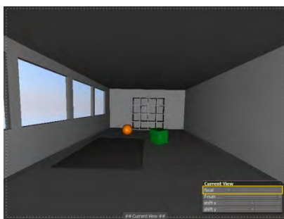
Figure 3-187: Small Focal Length (at 11 mm) creates a “zoom out” effect, though for too small values this can lead to unrealistic results.
