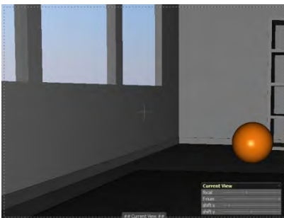
Figure 3-193: By dragging the bar leftwards, camera is shifted leftwards in X direction by -20 mm (at our example image)
