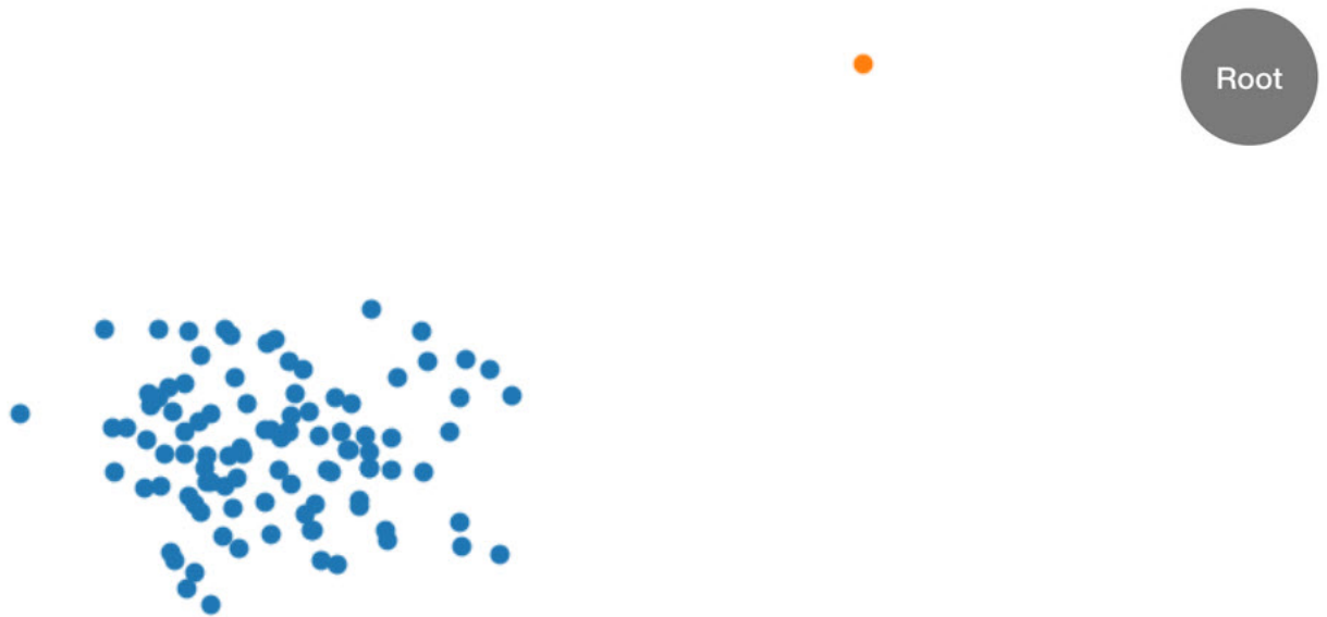
Figure 1. A two-dimensional dataset where the majority of data lies in a cluster (blue) except for one anomalous data point (orange). The tree is initialized with a root node.
